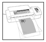
Remove your material from the support tray after it has cleared the exit (a). If you are finished with the job, but plan to use the laminator again soon, press start 11 to put it into the **standby mode**. If you forget, it will switch itself into this mode after one hour of inactivity. Press start 11 again to resume work, or press the power button (2) to turn off the machine.
